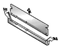
Figure 9-7. Removing a DIMM
