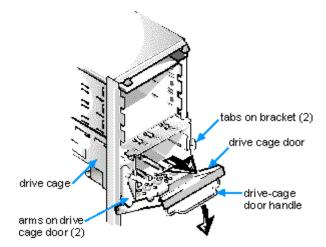
Figure 10-10. Removing the Hard-Disk Drive Bracket
