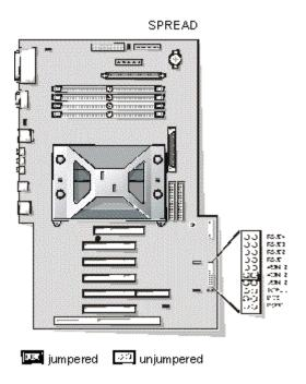
Figure B-1. System Board Jumpers
