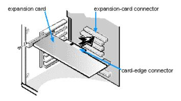
Figure 9-4. Installing an Expansion Card
