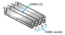
Figure 9-5. DIMMs and DIMM Sockets
