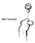
Figure 9-3. Removing the Filler Bracket
