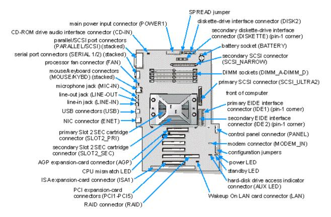
Figure 9-1. System Board Features
