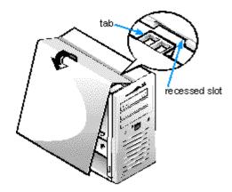
Figure 8-3. Replacing the Computer Cover
