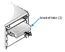
Figure 10-6. Removing a Drive
