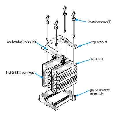
Figure 9-8. Slot 2 SEC Cartridge/Heat Sink Assembly Removal
