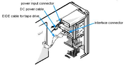
Figure 10-9. Attaching EIDE Tape Drive Cables
