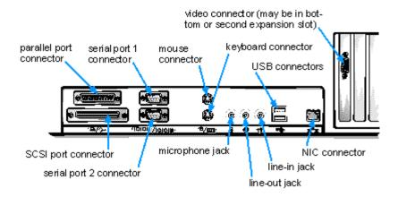
Figure B-2. I/O Ports and Connectors
