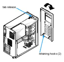
Figure 10-2. Removing the Front Bezel
