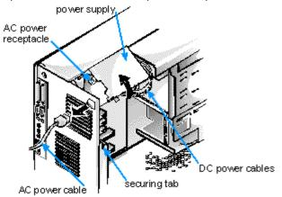
Figure 8-6. Rotating the Power Supply
