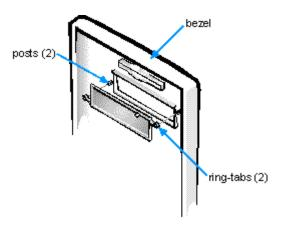
Figure 10-3. Removing the Front-Panel Insert for a 5.25-Inch Bay
