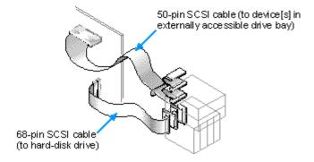
Figure 10-14. Internal SCSI Cable
