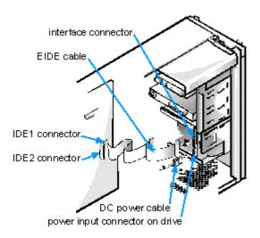
Figure 10-13. Attaching Hard-Disk Drive Cables
