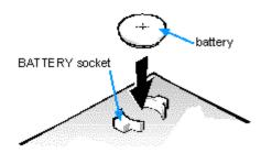
Figure 9-9. System Battery and Battery Socket
