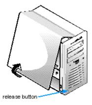
Figure 8-2. Removing the Computer Cover
