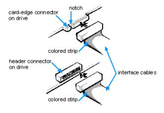
Figure 10-5. Drive Interface Connectors
