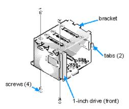
Figure 10-11. Inserting a 1-Inch Hard-Disk Drive Into the Bracket
