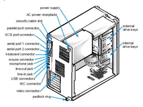
Figure 8-5. Inside the Chassis
